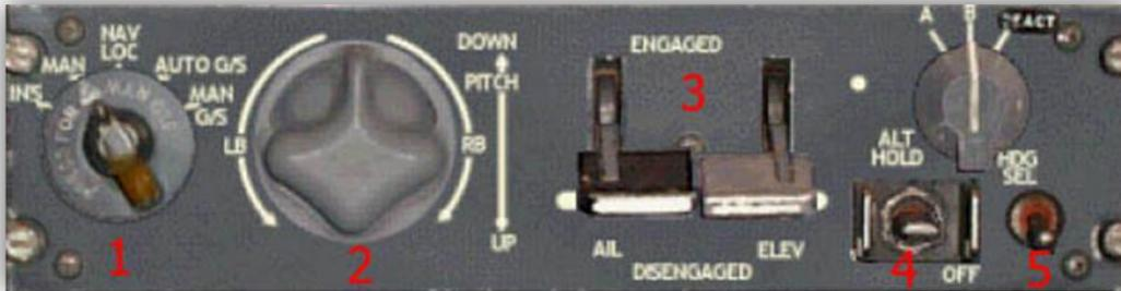
The Autopilot control unit is located in the radio stack, lower right side of the captain. There are 2 knobs, 2 levers and 2 switches that operate the SP-50.
